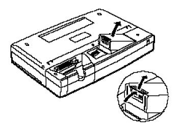
3. Lift the battery pack out of the battery compartment.
